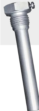
THR -VA-17 / xx Immersion sleeve, stainless steel V4A (1.4571) flat sealing, cylindrical, according to DIN 228
