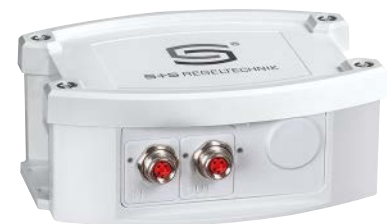
EtherCATP Cable connection and LED status display
